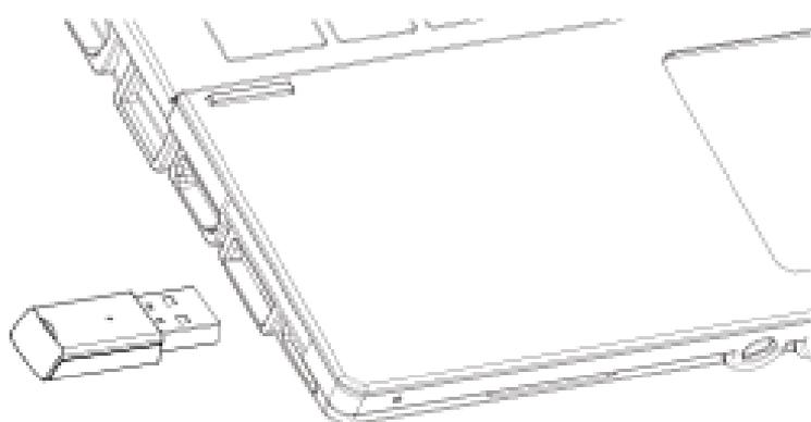
(The USB receiver into the computer USB port)
